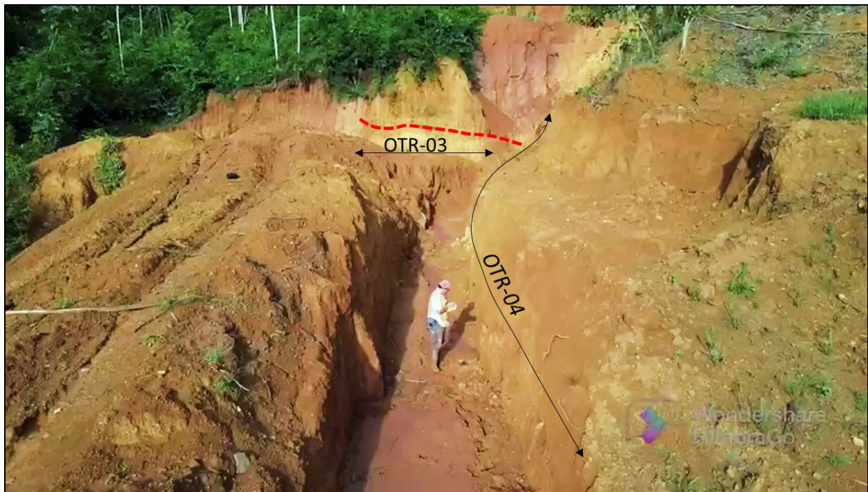
FIGURE 9.15 OTR-03 AND OTR-04 SAMPLE LOCATION LOOKING EAST, MAIN QUARTZ VEIN IN RED DOTTED LINE
