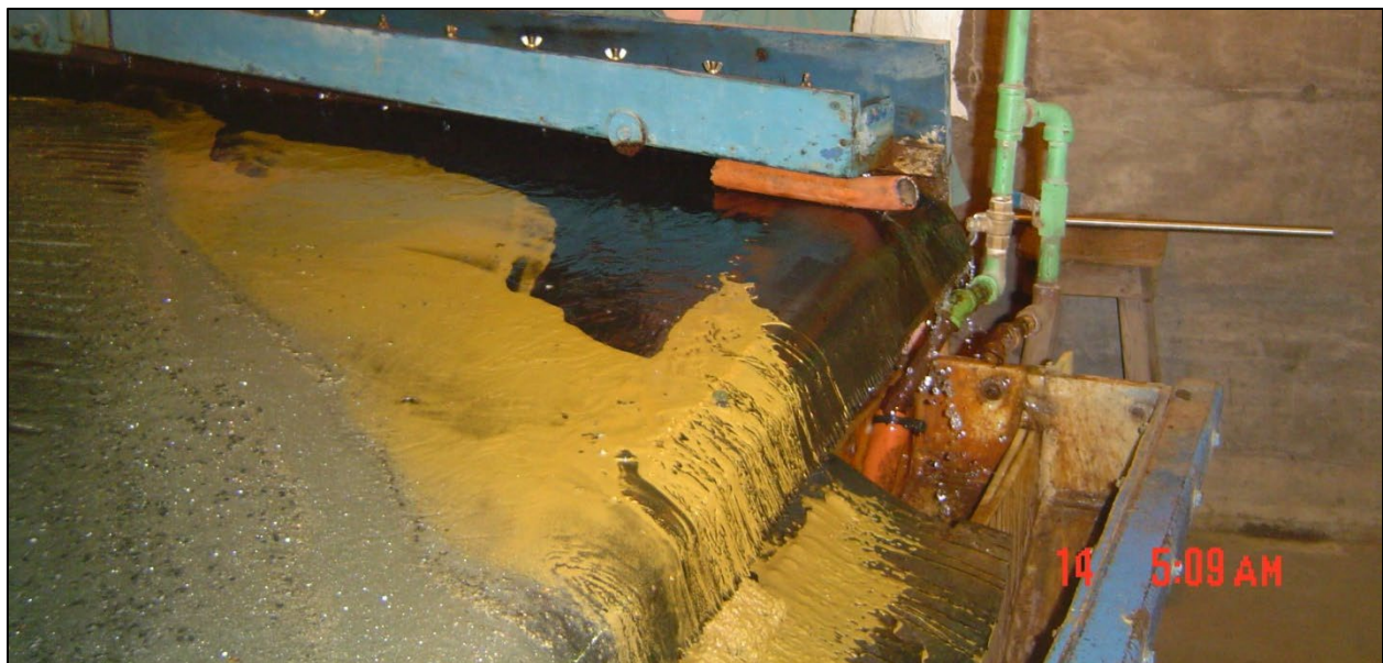
FIGURE 13.2 GOLD CONCENTRATION ON SHAKING TABLE 1
